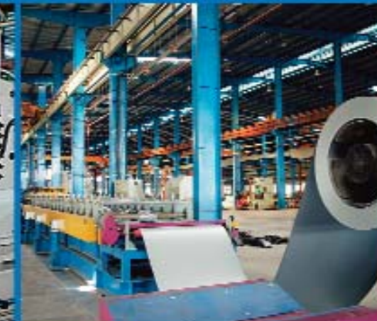
Roof & wall sheeting machine - finishing side M/s ILKWANG - KOREA
